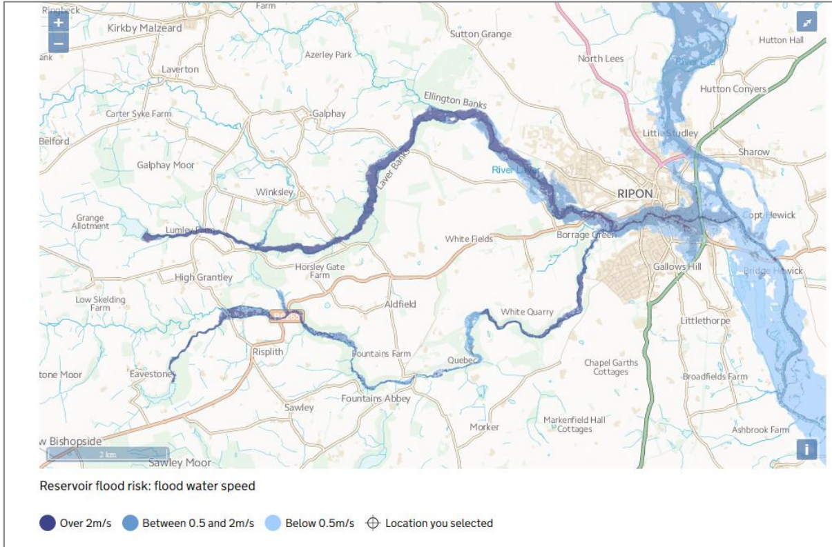
Figure F4 Flood water speed from example small reservoirs
