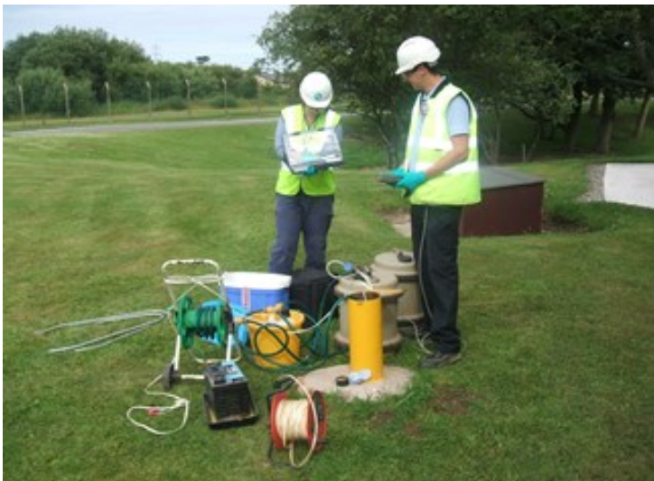
Figure 3. Groundwater Monitoring at Chapelcross
