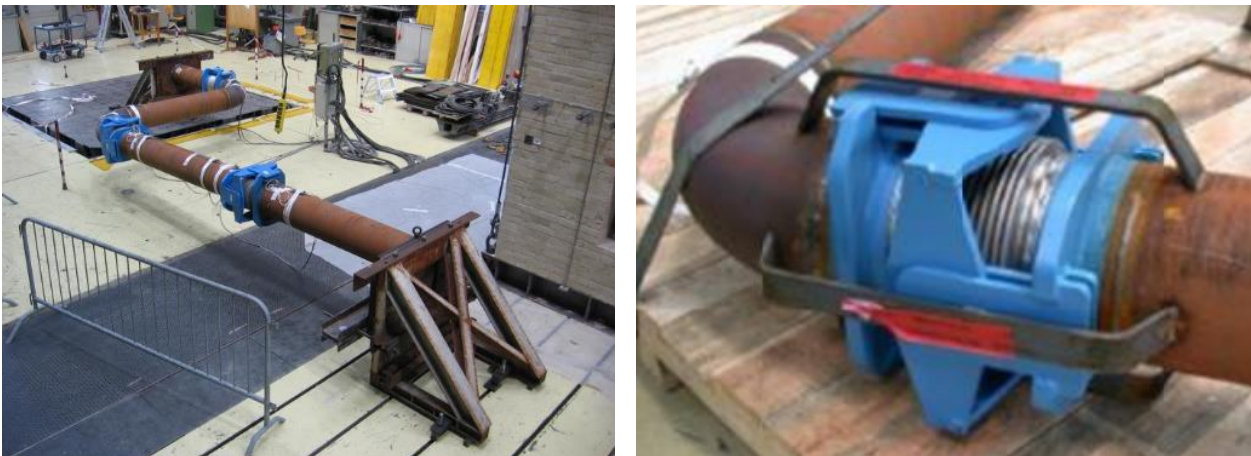
Figure 10 Pipeline expansion joints (ambient temperature and pressure) used for seismically isolated tanks in petrochemical plants [34] [41]
