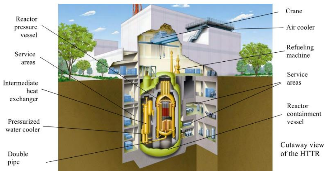
Figure 3 Cut-away of HTTR showing deep embedment of an AMR [8]
